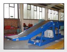
A power boom feeder fitted at the rear of the vehicle loader offers increased flexibility when loading product onto the machine.
