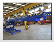
Our mobile vehicle loaders are ideal for loading and unloading vehicles without a loading bay or raised dock.
